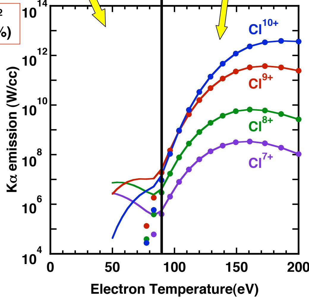
Emission density of K $\alpha$ -radiations is very small in comparison with that by fast electrons generated by sub-ps laser pulses.
