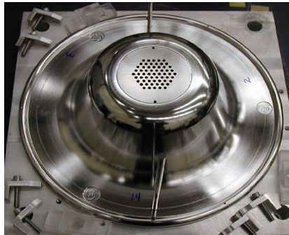
High Gradient Insulators held 30 kV/cm
