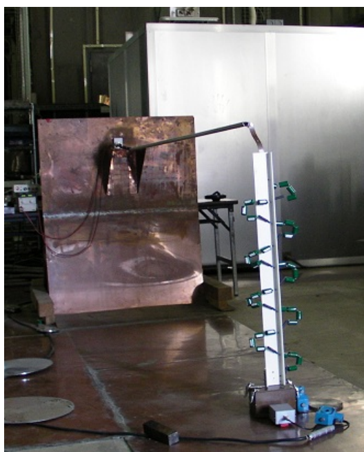
Fig. 3 Setup of Step Response Measurement and Divider
